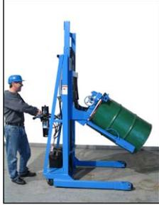
3. Tilt drum to horizontal and transport to racking location
