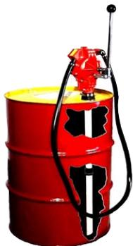
The self priming piston pumps on the forward and back strokes to yield a gallon in fewer than five cycles. Use for liquids at temperatures up to 80° F (25 C) and maximum viscosity of 2,000 SSU (e.g. 30W motor oil). Each pump is compatible with specific chemicals. Check Morse website for chemical compatibility of each liquid by chemical name. It is the user's responsibility to take appropriate safety and protective measures with hazardous chemicals.
