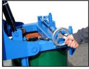
1. Manually secure clamp to grip drum
